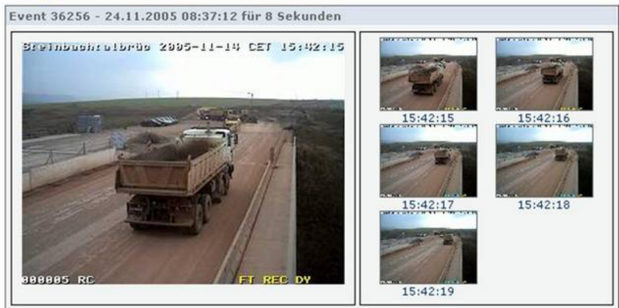
Figure 5 Monitoring system set up to act securing photographical evidence. Shown are the pictures taken from a web camera, which is triggered by strain measurements.
