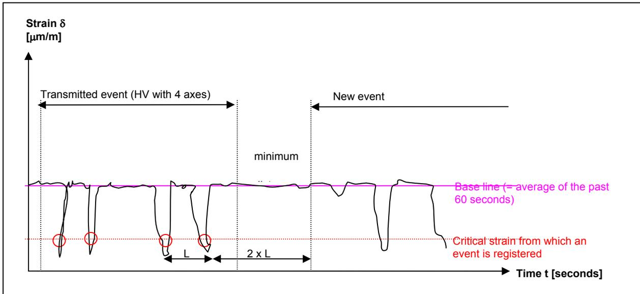
**Fig. 6.** Principle of dynamic recognition of a truck on the expansion joint (theoretical model).
