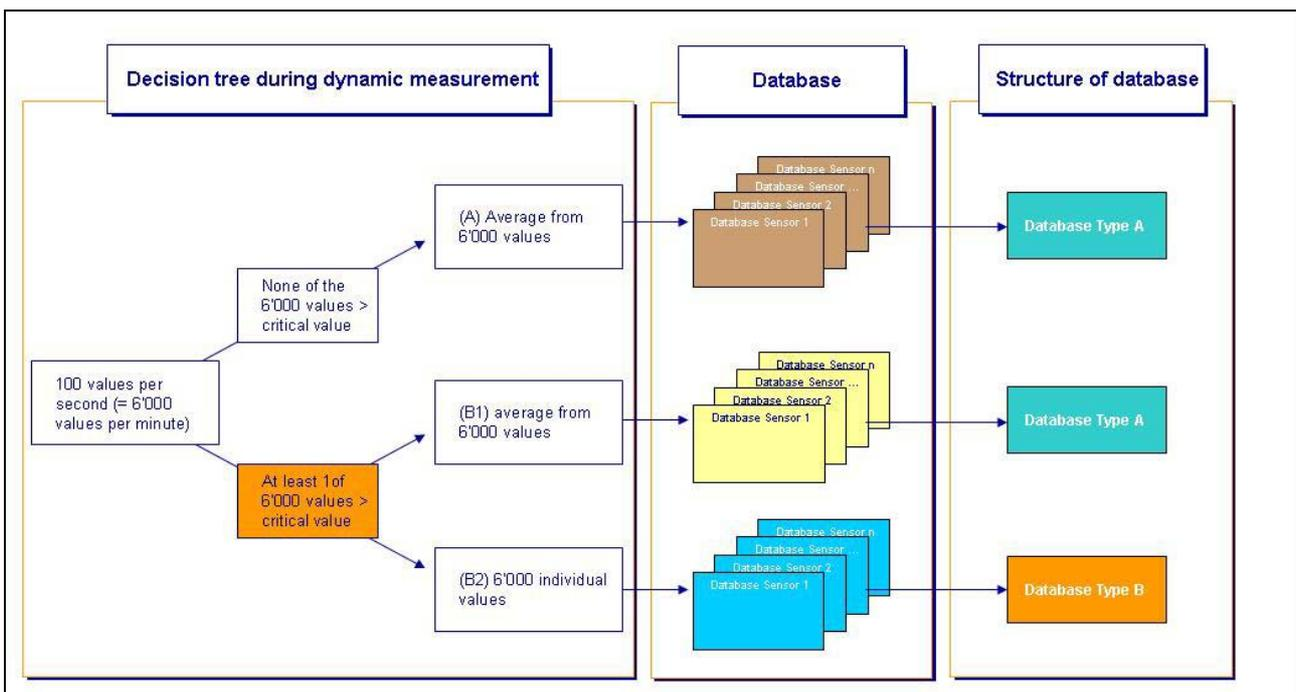
**Fig. 5.** Configuration and arrangement of the database enables a clear presentation of data
